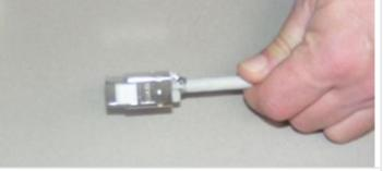
The finished connector should not show any wires at the
