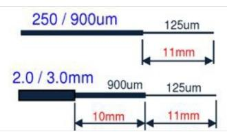
Slide on correct boot, and screw cover. Prepare fiber as below. Strip and clean it. Cleave fiber precisely.
