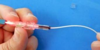
Form a small curve. Then, press metal Button to connect fibers. You will see no leakage of red light for a low loss
