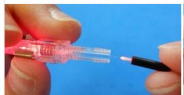
Insert fiber to LC Connector until it touches the fiber inside.
